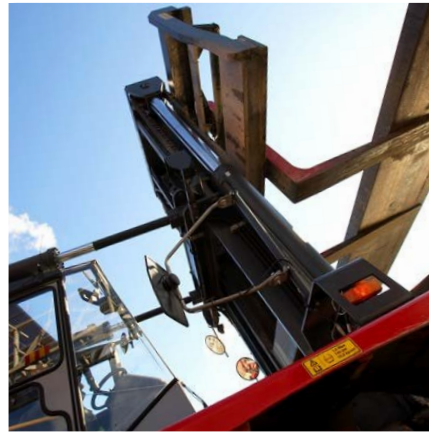
Full visual contact with the load and attachment, is provided by the Spirit Delta cabin and the open design of the mast and carriage.
