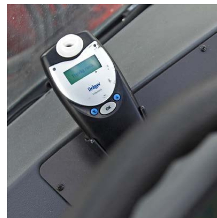
To increase workplace safety the machine can be fitted with alcohol interlock.
